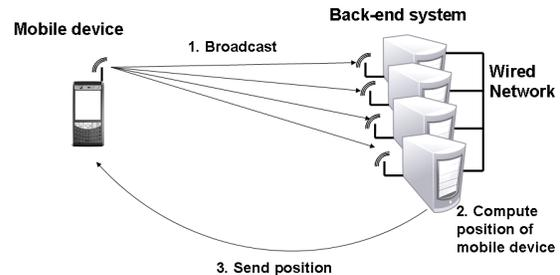
Fig. 2. Distributed Positioning: The back-end systems distributively estimates the position of the mobile device based on data transmitted from the device.
