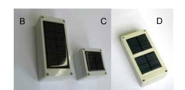
P<sub>max</sub>=405mW I<sub>max</sub>=81mA V<sub>max</sub>=5V
