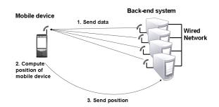
Fig. 1. Self Positioning: The mobile device estimates its position based on data transmitted from the back-end system.
