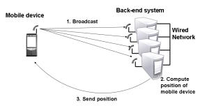
Fig. 2. Distributed Positioning: The back-end systems distributively estimates the position of the mobile device based on data transmitted from the device.
