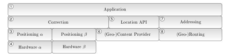
Fig. 3. Layered architecture for indoor location based services.
